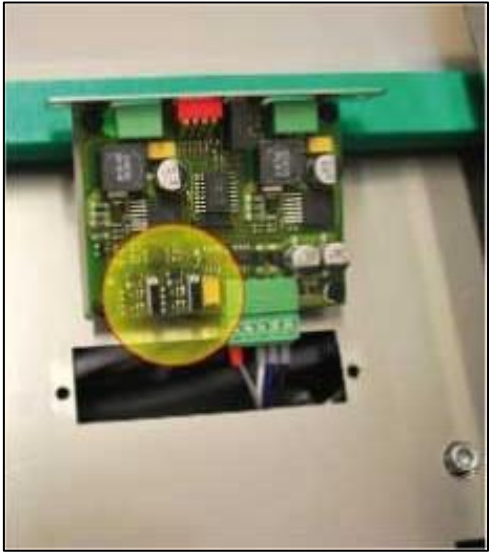
Figure 6-6: Switches on LED Controller
